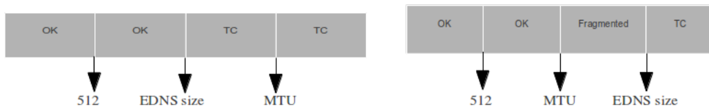
Figure 1: Effect of response size on its status over UDP
